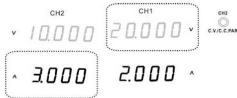
Slave (CH2) voltage level: CH1 meter reading shows the output voltage. In the above case, 20.0V.
