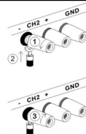
Banana plug Insert the plug into the socket.
