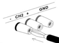
Wire type When using load cables other than the attached, make sure they have enough current capacity for minimizing cable loss and load line impedance. Voltage drop across a wire should not exceed 0.5V. The following list is the wire current rating at 450A/cm<sup>2</sup>.
