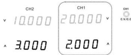
Voltage level: The CH1 meter reading shows the output voltage. In the above case, 20.0V.
