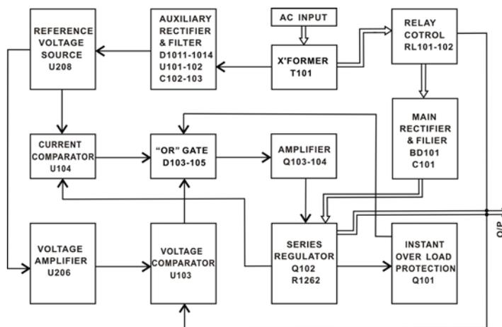
Rectifier The auxiliary rectifiers D1011~D1014 provide bias voltage filtered by the capacitors C102 and C103, for the pre-regulators U101 and U102. They provide a regulated voltage for other modules.
