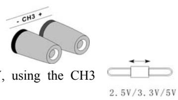
2. Select the output voltage from 2.5V, 3.3V and 5V, using the CH3 voltage selector switch.
