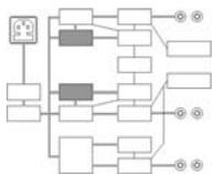
The AUX power for Channel 1 and 2 produces the power source for auxiliary devices, such as analog/digital controller, relay, LED display, and cooling fan. Altogether four pairs of power source are generated for different purpose: ±12V, +5V, and +12 V.
