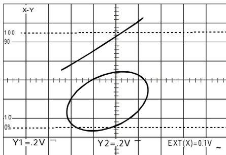
Figure 5-8 Typical dual X-Y display
